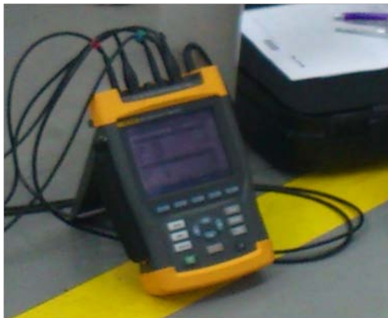
Figure 3. Fluke power quality meter.
