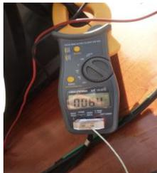
**Picture 4.** Multimeter measuring a cell temperature of 64°C in a sunny day with 28°C of outside temperature.
