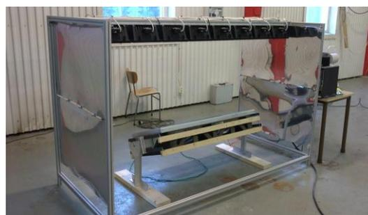
**Picture 2.** The solar simulator for the indoor measurements.
