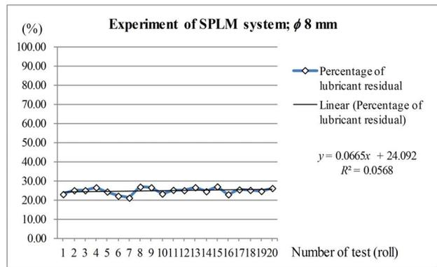
Figure 13. Oil residual in φ 8 mm copper pipe using SPLM.
