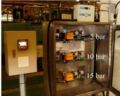
Figure 4. Pressure control system for industrial factory.
