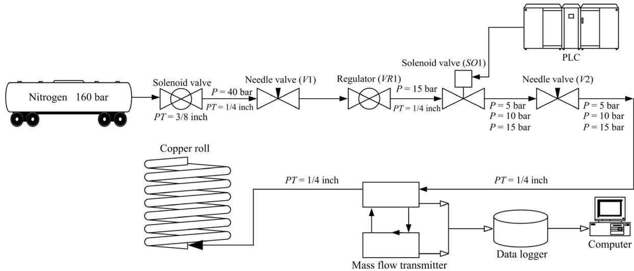
Figure 5. Diagram of serial pressure ladder module (SPLM).
