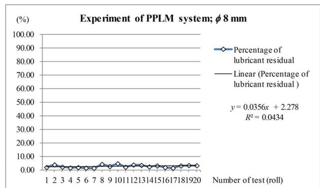
**Figure 9. Oil residual in  $\phi$ 8 mm copper pipe using PPLM.**
