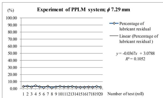
**Figure 8. Oil residual in  $\phi$ 7.29 mm copper pipe using PPLM.**
