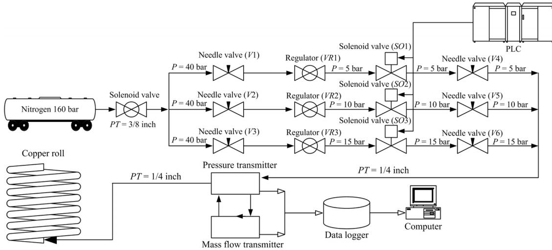
Figure 3. Diagram of parallel pressure ladder module (PPLM).
