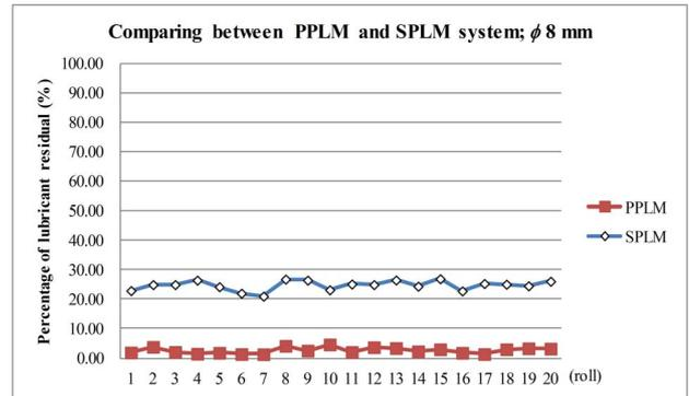
Figure 14. Oil residual in  $\phi 7.29$  mm copper pipe were compared between using PPLM and SPLM system.
