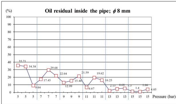
Figure 11. A appropriate pressure testing, φ 8 mm.
