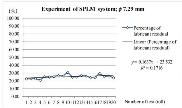
Figure 12. Oil residual in φ 7.29 mm copper pipe using SPLM.
