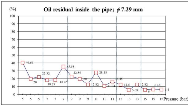
Figure 10. A appropriate pressure testing, φ 7.29 mm.
