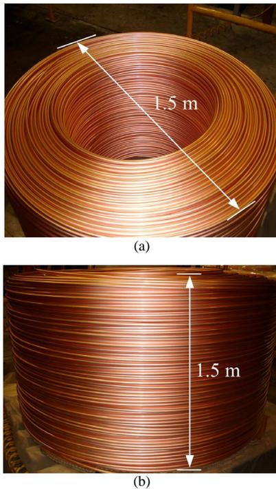
**Figure 1. Copper roll after ironing process. (a) Top view; (b) Side view.**
