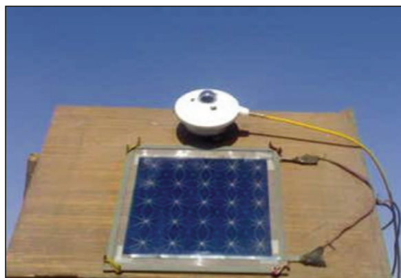
Figure 1. Multicrystalline silicon solar cell in the outdoor located at optimum tilt angle with the radiation sensor.
