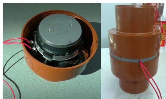
Figure 5. The enclosure housing linear alternator.
