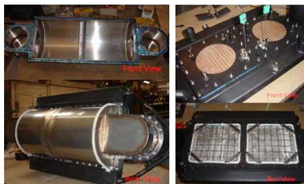
Figure 2. Radiant bulge hot heat exchanger (left); Ambient heat exchanger (right).
