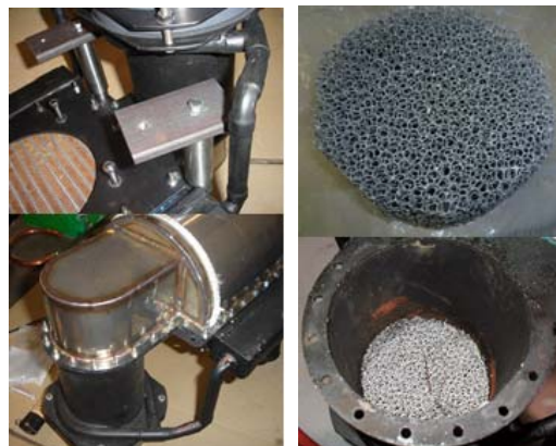
Figure 3. Thermal buffer tube (left); Secondary ambient heat exchanger (right).
