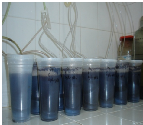
Figure 6. System used in the aerated biological treatment.
