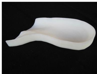
**Figure 5.** Prototype of customized orthosis fabricated.
