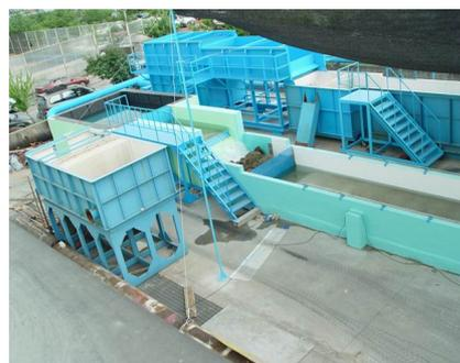
Figure 2. Experiment flume and water supply.
