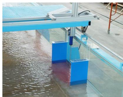
Figure 3. Experiment setup of groynes for  $L/l = 2$ .
