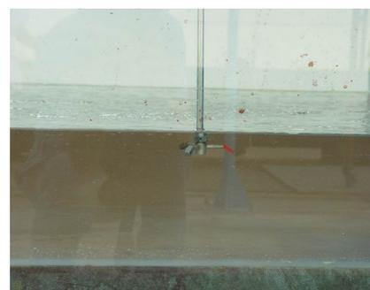
Figure 4. Measurement of velocity using ADV.
