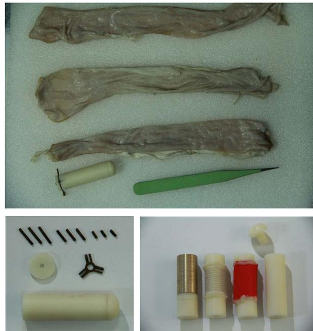
**Figure 4. Pig small intestine sample used in test (top). Micro robot model with adjustable legs (bottom left). Models used in material-tension test (bottom right).**
