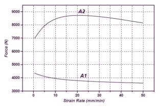
Figure 13. Variation of force versus strain rate of A2 and A1 sample.
