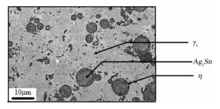
Figure 7. SEM micrograph of A1 sample.
