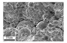
Figure 11. SEM micrograph of fracture surface of A2 sample.
