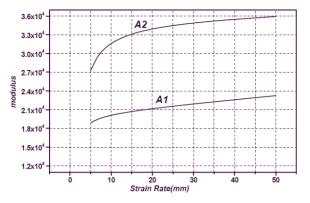
Figure 15. Variation of modulus versus strain rate as a function of copper.
