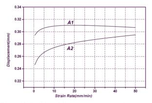
Figure 14. Variation of displacement versus strain rate as a function of Cu.
