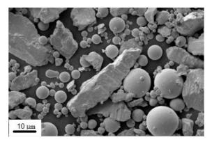
Figure 1. SEM micrograph of admixed high copper amalgam.
