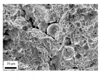
Figure 12. Crack propagation in A1 sample.
