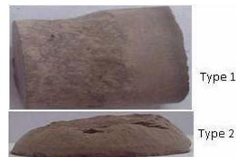
**Figure 2.** Fractures of the compacted powder after ejection.
