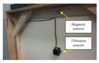
Figure 12. Final position of vibration and magnetic sensors.
