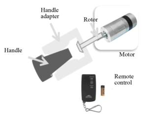
Figure 16. Scenario of lock/unlock the door via remote control.
