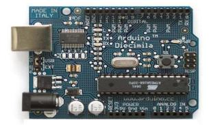
Figure 9. Arduino microcontroller board.
