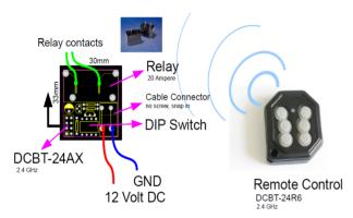
Figure 6. Detailed characteristics of the relay receiver board with remote control.
