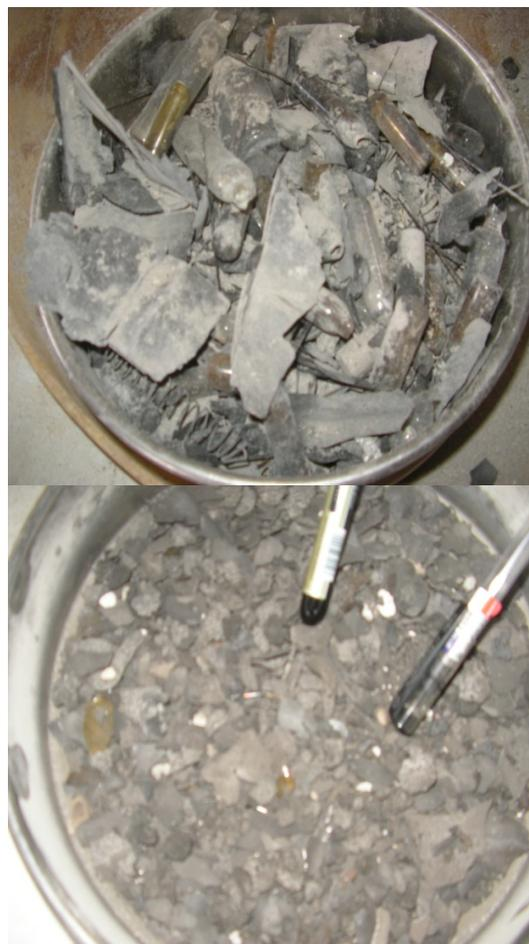
**Figure 2.** Non-combustible materials from incinerator ash before and after sieving.
