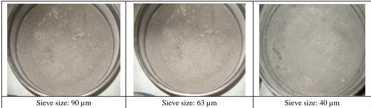
Figure 3. Ashes from incinerator after sieving at different sizes.
