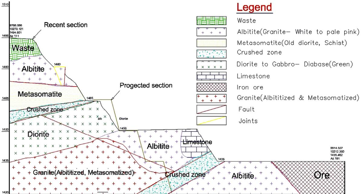
Figure 2. The geological profile perpendicular on the west wall of Chadormalu iron ore mine.
