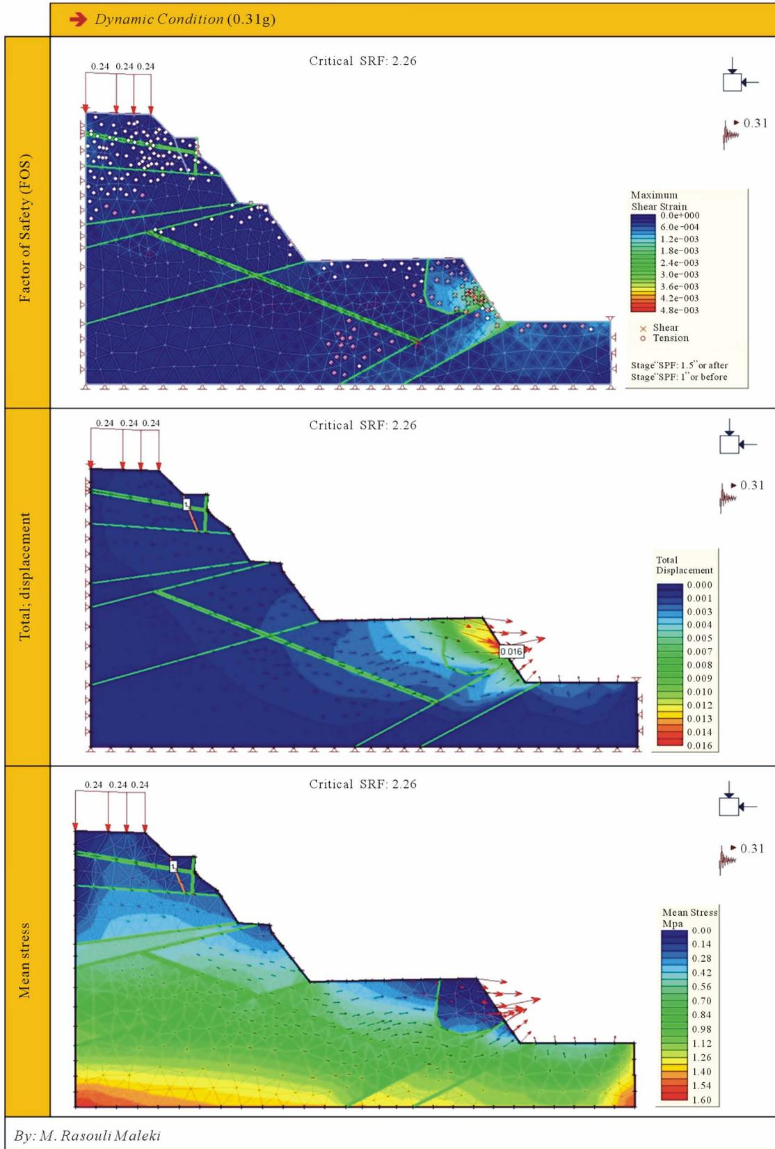
Figure 3. Output model of Phase2D software, factor of safety (FOS), total displacements and mean stress for static state.
