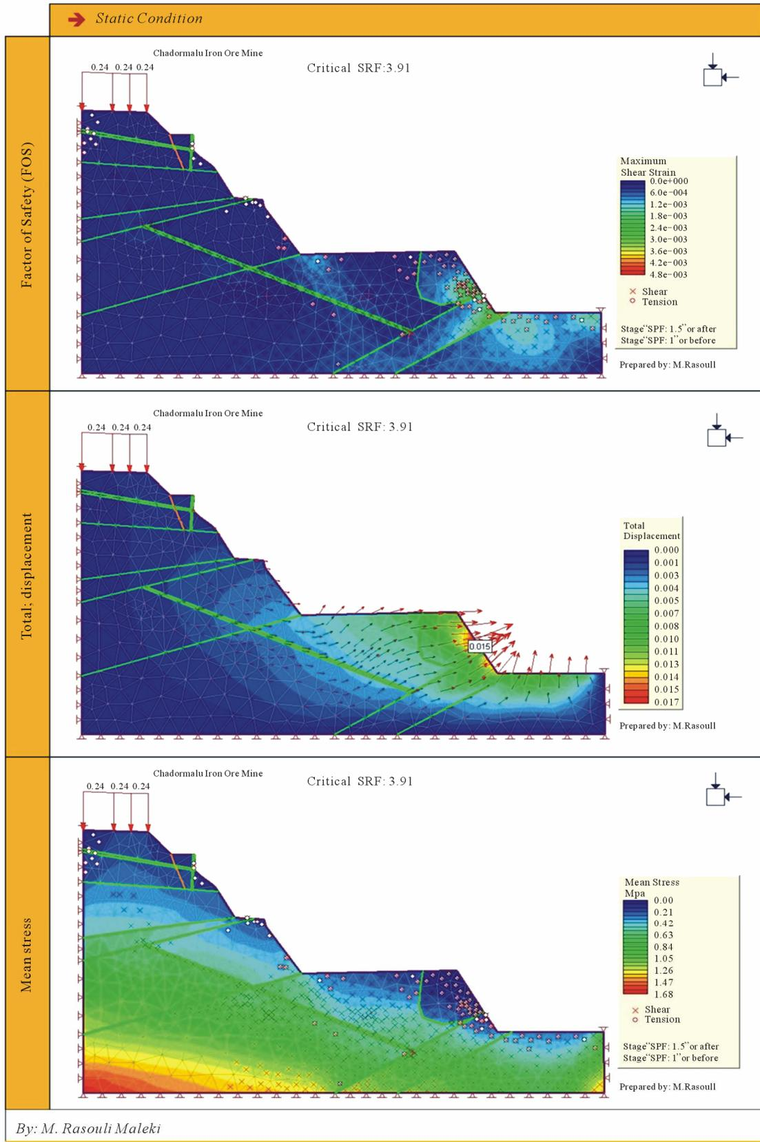
Figure 4. Output model of Phase2D software, factor of safety (FOS), total displacements and mean stress for dynamic state.
