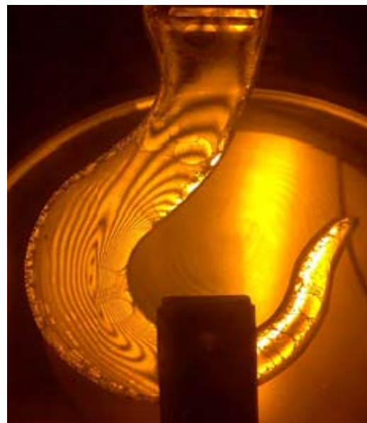
Figure 3. stress pattern of photo elastic model under sodium light.
