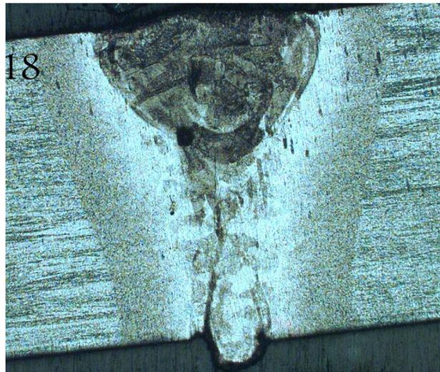
$$P = 1.7 \text{ mm}; W_{fz} = 1.319 \text{ mm}; W_{haz} = 2.087 \text{ mm}; \\ A_{fz} = 1.2508 \text{ mm}^2; A_{haz} = 1.8655 \text{ mm}^2$$
