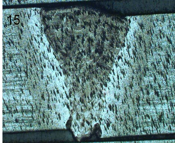
$$P = 1.65 \text{ mm}; W_{fz} = 1.357 \text{ mm}; W_{haz} = 2.190 \text{ mm}; \\ A_{fz} = 1.5909 \text{ mm}^2; A_{haz} = 1.6757 \text{ mm}^2$$
