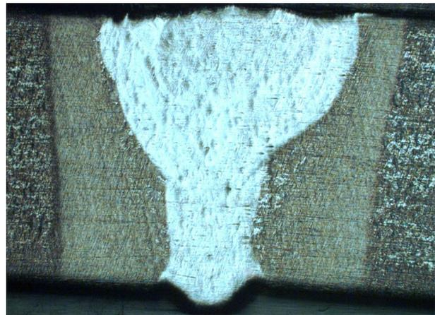
**Figure 2. Cross section of bead at optimum setting.**
