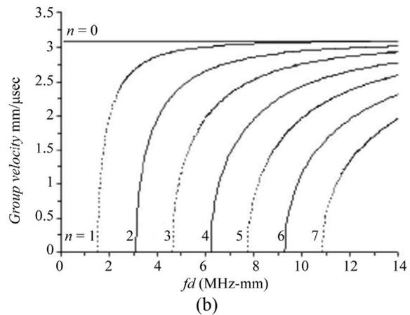
**Figure 5. Shear waves dispersion curves for stainless steel plate with thickness 5.89 mm. (a) phase velocity (mm/μsec); (b) group velocity (mm/μsec).**
