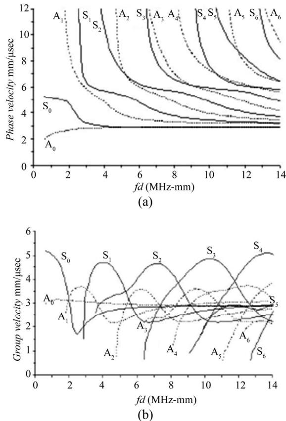
**Figure 6.** Lamb waves dispersion curves for stainless steel plate with thickness 5.89 mm. (a) phase velocity (mm/μsec); (b) group velocity (mm/μsec).
