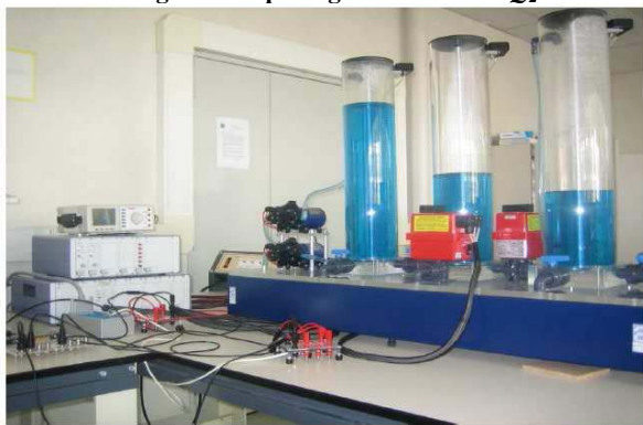
Figure 8. Real system. The parameters for both controls for three tanks are: \lambda = 0.6 , k_1 = 0.46 , k_2 = 0.32 , K_{11} = 10^{-3} , K_{12} = 3 \cdot 10^{-4} , K_{21} = 11 \cdot 10^{-5} and K_{22} = 7 \cdot 10^{-4} .
