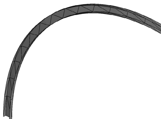
Figure 22. ABAQUS modeling of a mono-symmetric curved cantilever with shell elements.
