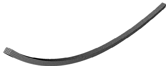
Figure 19. ABAQUS modeling of a 45 degree bend with solid elements.
