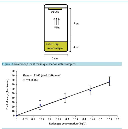
Figure 3. Shows the relation between radon gas concentration and track density in standard water samples.
