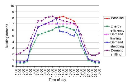
Figure 1. Examples of load shapes, this chart is conceptual; the data are not from actual measurements [9].
