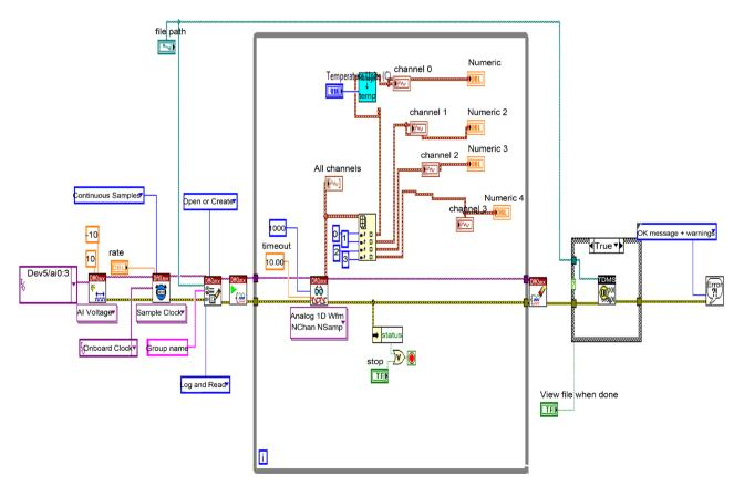
Figure 5. Multichannel DAQP using LabVIEW G code.
