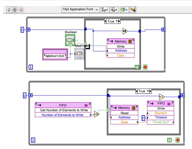
Figure 9. Design of FPGA target.vi for multichannel DAQP using LabVIEW G-code.
