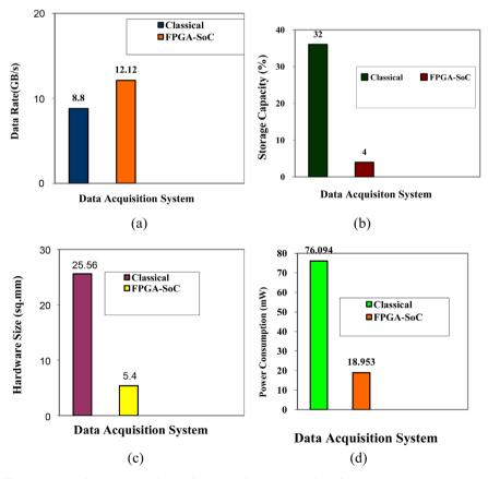
**Figure 12.** Performance analysis of proposed FPGA-SoC based DAQ system (a) Data rate speed (b) Storage capacity (c) Hardware size (d) Power consumption.
