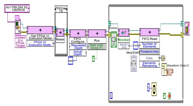
Figure 10. LabVIEW G-code for FPGA host.vi.
