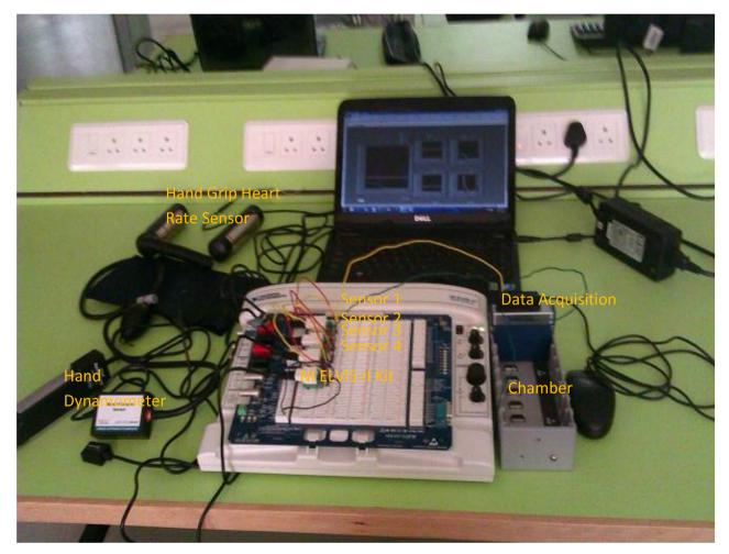
Figure 4. Experimental setup of multichannel DAQP.
