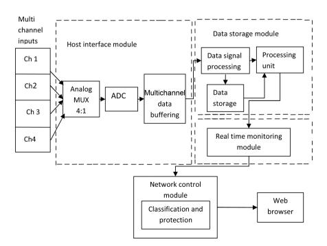
Figure 1. Multichannel DAQP module with network control module.
