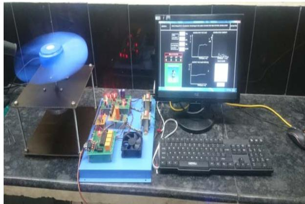
**Figure 11.** Experimental setup generator running condition with air blower.
