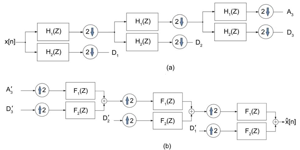
**Figure 2.** 3-level wavelet implementation. (a) Decomposition; (b) Reconstruction.
