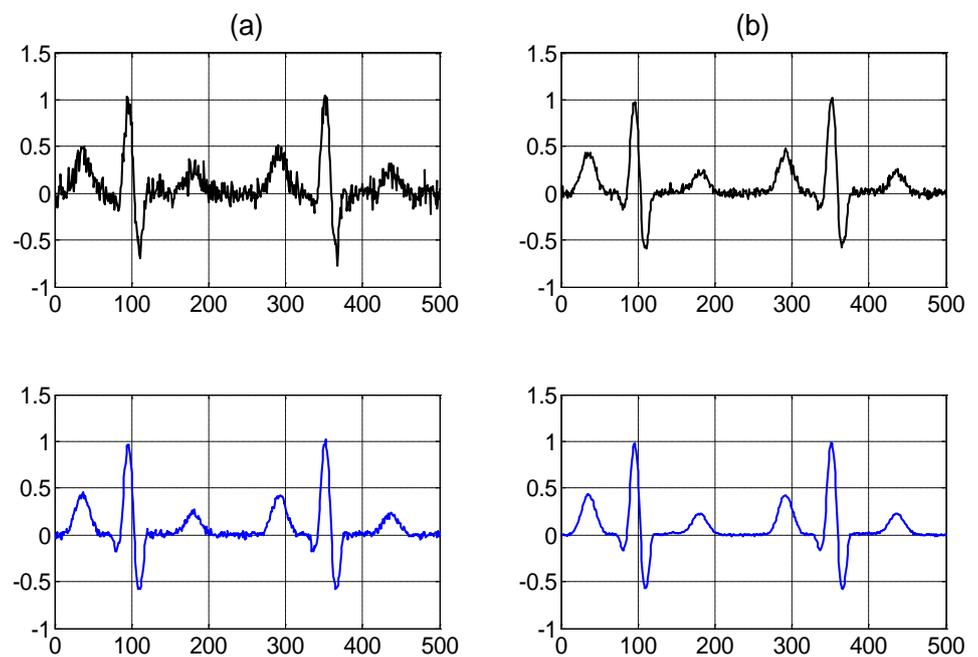
**Figure 3.** (a) The noisy and de-noised signal using proposed method (input SNR = 36.7 dB and output SNR = 48.7 dB) and (b) noisy and de-noised signal using proposed method (input SNR = 45.2 dB and output SNR = 59.2 dB).
