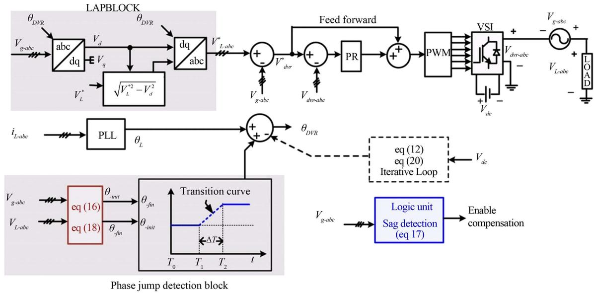
**Figure 3.** Detailed block diagram of the proposed phase Skip compensate on method with LAP injection. (Cited from Power Electronics Converters, Applications and Design (Wiley, 2003)).
