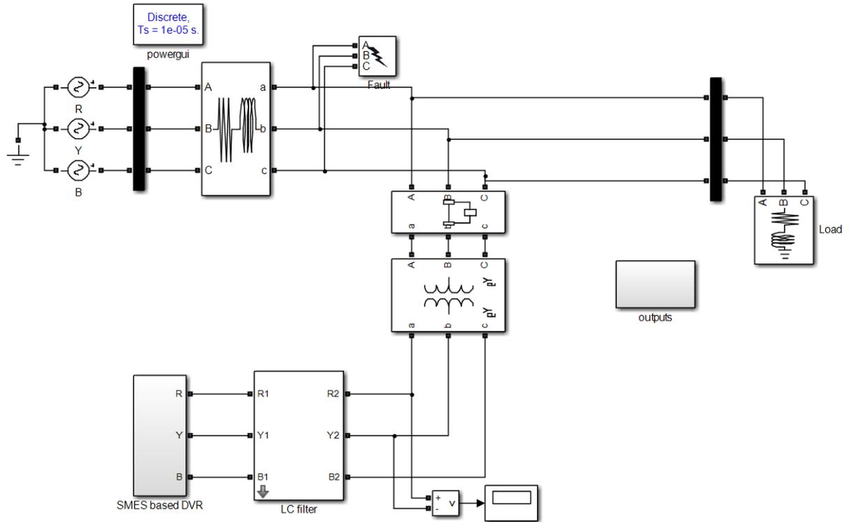
**Figure 6.** DVR connected at the distribution end near fault.
