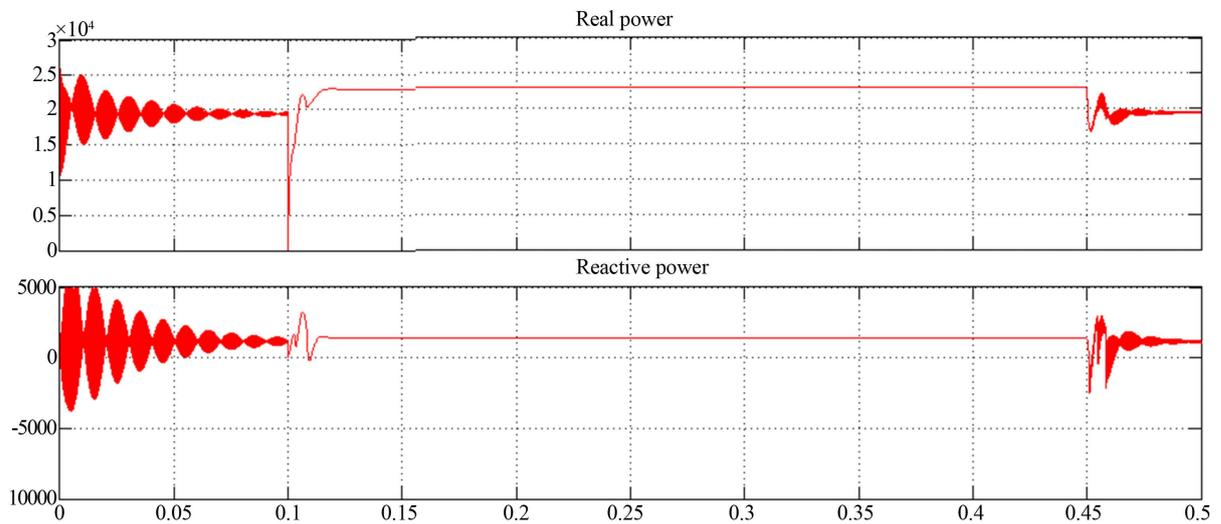
Figure 12. Real and Reactive power after SMES based DVR and ODFD control.
