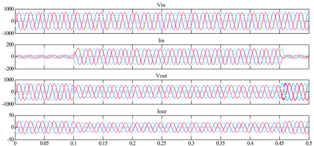
Figure 10. Voltage and Current waveforms without SMES based DVR.
