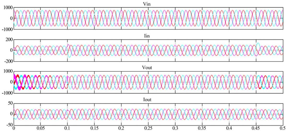
Figure 11. Voltage and Current waveform with SMES based DVR and ODFP control.
