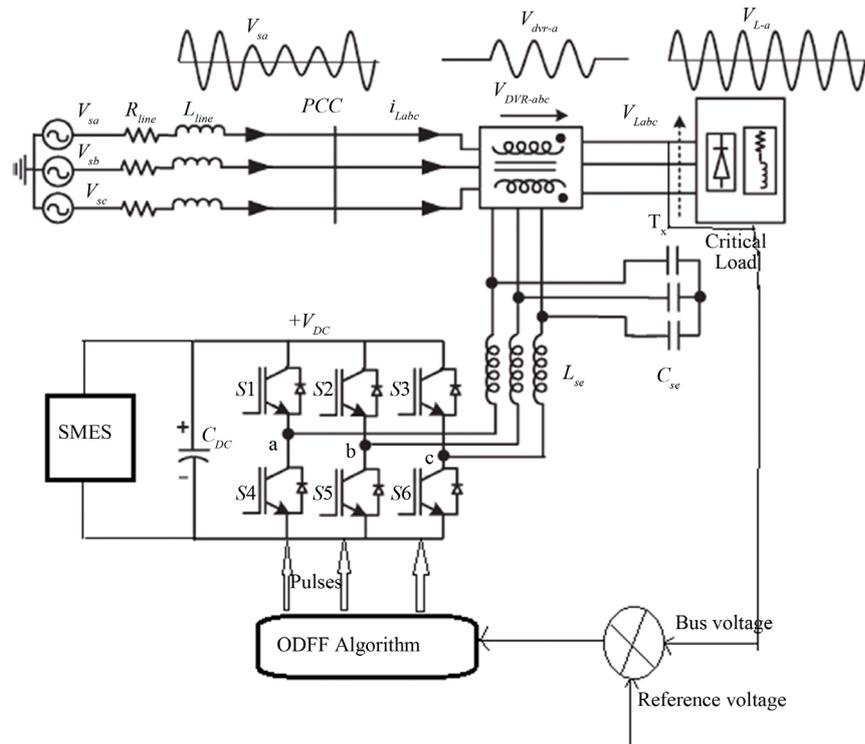
Figure 1. Proposed architecture. (Cited from SRF theory revisited to control self-supported dynamic voltage restorer (DVR) (P. Kanjiya, 2013)).
