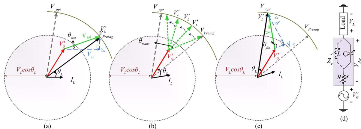
Figure 2. Phasor diagram for the proposed sag compensation method. (a) Presag restoration, (b) intermediate transition, (c) final load voltage with LAP injection, and (d) SMES based DVR visualization as the variable virtual impedance changes from resistive to dominant capacitive (for sag) or inductive (for swell). (Cited from Voltage Sag Compensation Scheme for Dynamic Voltage Restorer (Rauf, 2015)).
