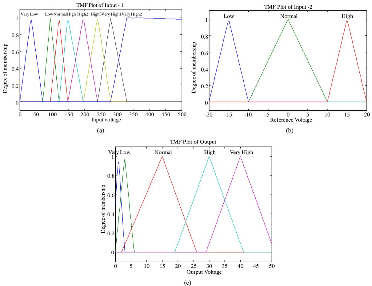
Figure 5. Input membership function for (a) Load voltage (b) Reference voltage and (c) Output membership function (Predicted Vsag) (Cited from Knowledge representation in fuzzy logic., (Zadeh, L.A., 1989)).
