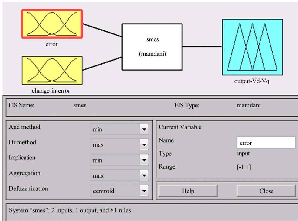
**Figure 8.** Fuzzy logic control references (Cited from Fuzzy logic Toolbox MATLAB. (2013 a)).
