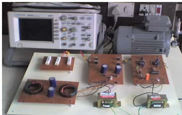
Figure 8. Reduced switch Z-source inverter-fed induction motor drive prototype.
