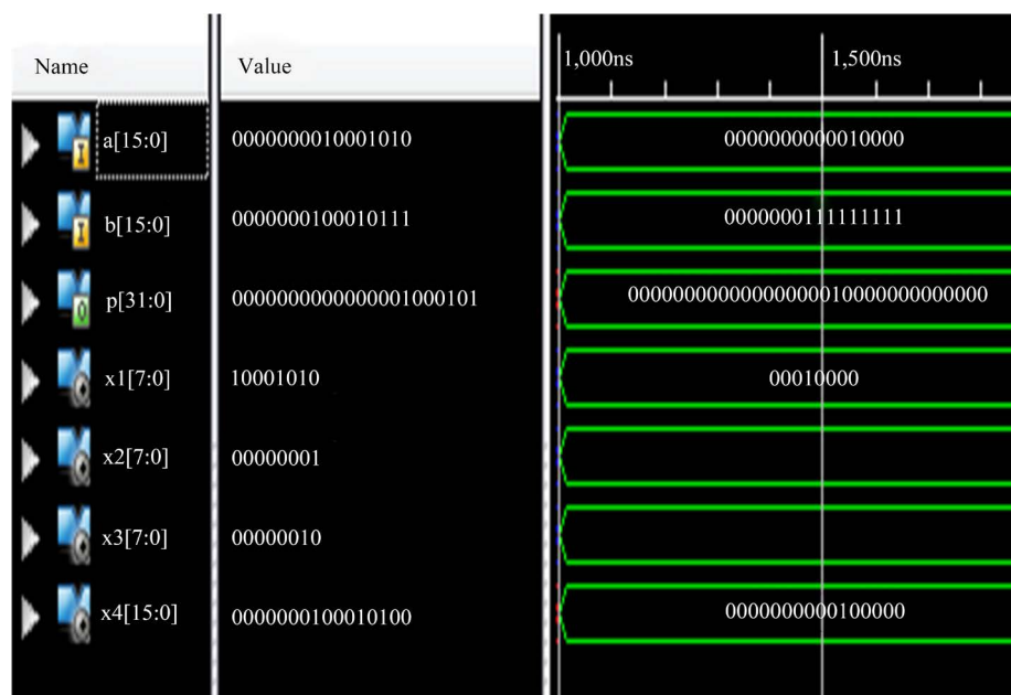
Figure 5. Simulation output of approximate multiplier.
