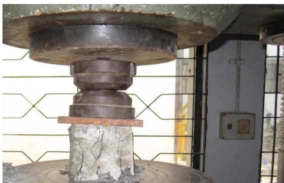
Figure 4. Compressive strength test.
