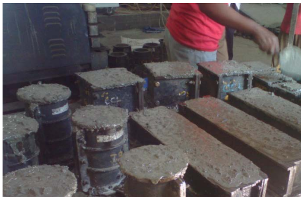
Figure 3. Casting of specimens.
