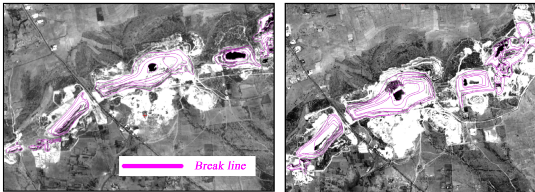
Figure 3. Volume derivation for the year 2006 (left) and 2014 (Right) using Leica Photogrammetry Suite.
