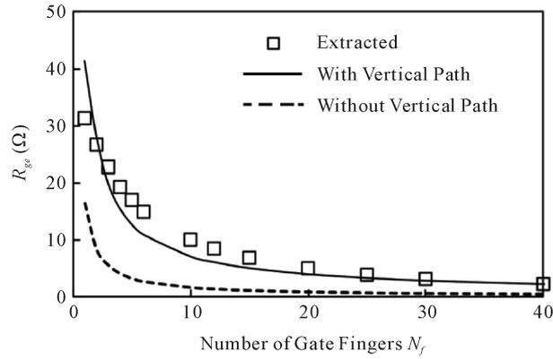
**Figure 3.** Extracted and calculated values of gate resistance  $R_{gs}$  versus the number of gate fingers  $N_f$  ( $L = 140$  nm,  $W_f = 3$   $\mu\text{m}$ , both-side gate connection).
