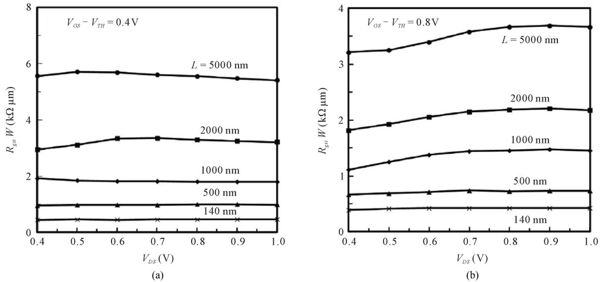
**Figure 4.** Extracted values of NQS gate-source resistance  $R_{gsi}$  of NMOS devices with gate length  $L = 140$ ; 500; 1000; 2000 and 5000 nm at gate-source overdrive voltages (a)  $V_{GS} - V_{TH} = 0.4$  V and (b)  $V_{GS} - V_{TH} = 0.8$  V (gate width is  $120$   $\mu\text{m}$  ( $3$   $\mu\text{m} \times 40$  fingers), both-side gate connection).
