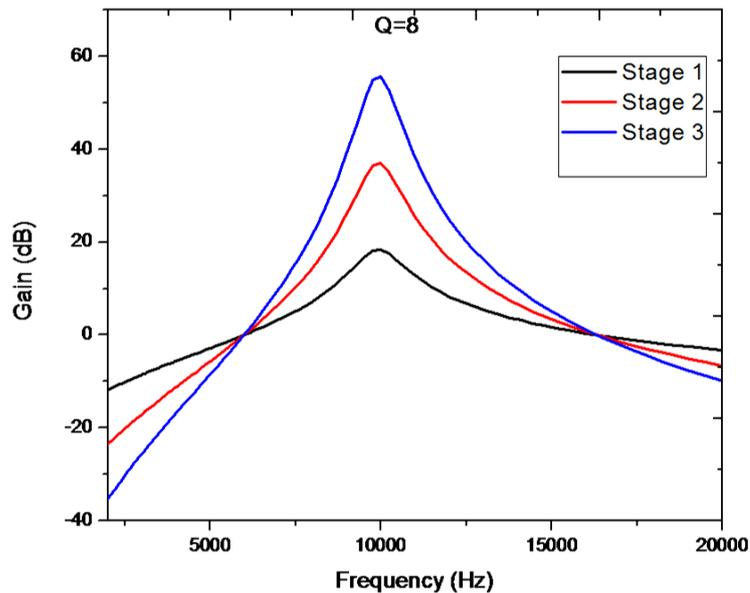
**Figure 3.** Cascaded R-filter sections (stages) magnitude response for  $Q = 8$ .
