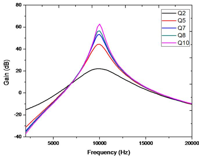
**Figure 4.** Cascaded band pass magnitude response of R-filter for different  $Q$ -values.
