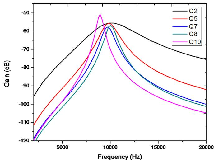
**Figure 5.** Cascaded band pass magnitude response of RC-filter for different  $Q$ -values.
