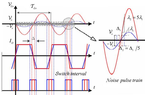
**Figure 9.** The influence of  $v_{LO}$  on  $\Delta$  and the resulting noise contribution.
