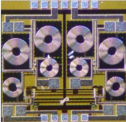
**Figure 8.** Microphotograph of the implemented DBGCC CAAB mixer.
