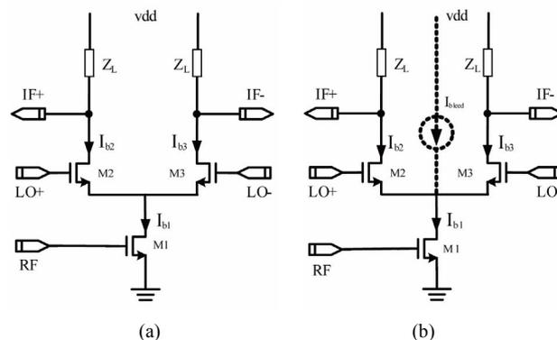
**Figure 1. Schematic of (a) Conventional single-balanced mixer; (b) Single-balanced mixer with current bleeding.**
