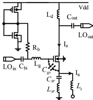
**Figure 4.** Topology of current bleeding source—Amp (class-A amplifier).
