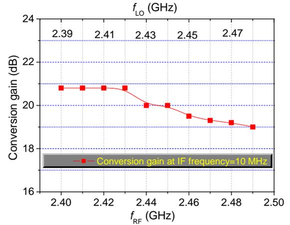
**Figure 16.** Conversion gain of the DBGC CAAB mixer versus frequency when IF frequency = 10 MHz.
