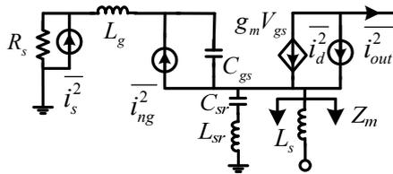
**Figure 5.** Equivalent circuits of the class-A amplifier (Amp) in **Figure 4**.
