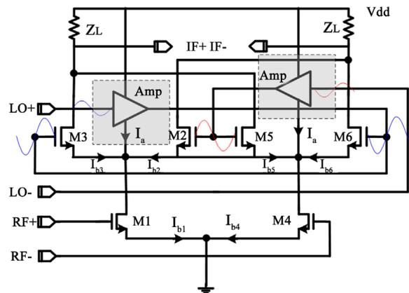
**Figure 3.** Schematic of DBGC CAAB mixer.
