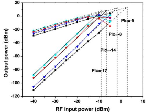
**Figure 14. IIP3 of the DBGCC AAB mixer at different LO level.**
