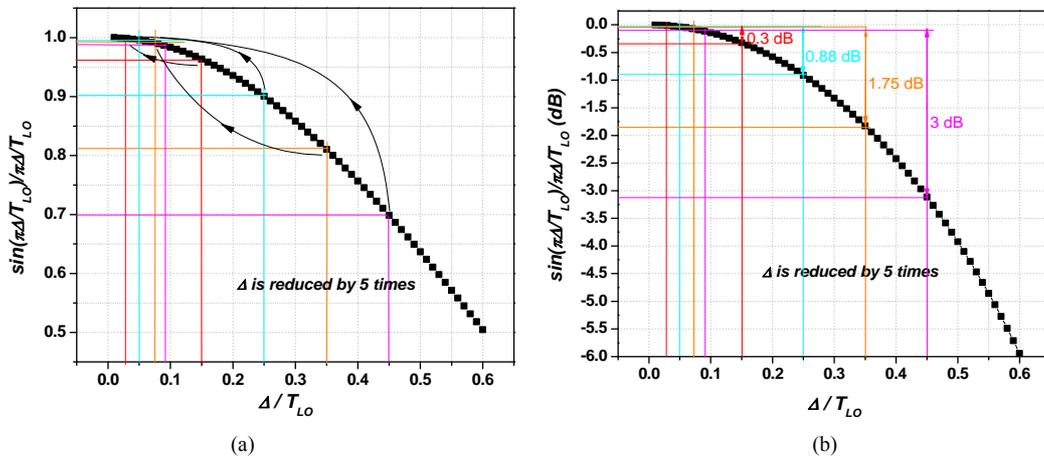
**Figure 11.** The switch loss reduction due to the switch interval  $\Delta$  shrinkage: (a) Linear scale; (b) Logarithm scale.
