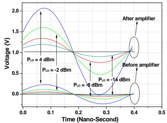
**Figure 7.** The voltage swing at the input and the output of Amp at varying input power level.
