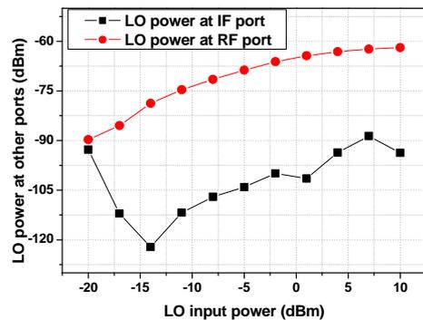
**Figure 15. LO power leakage to RF port and IF port.**
