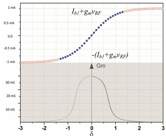
**Figure 2. I-V characteristic and equivalent transconductance of M2-M3, where  $\delta = v_{LO}/V_{od}$ .**
