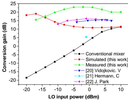
**Figure 12. The conversion gain comparison between the DBGCC AAB mixer and other works.**
