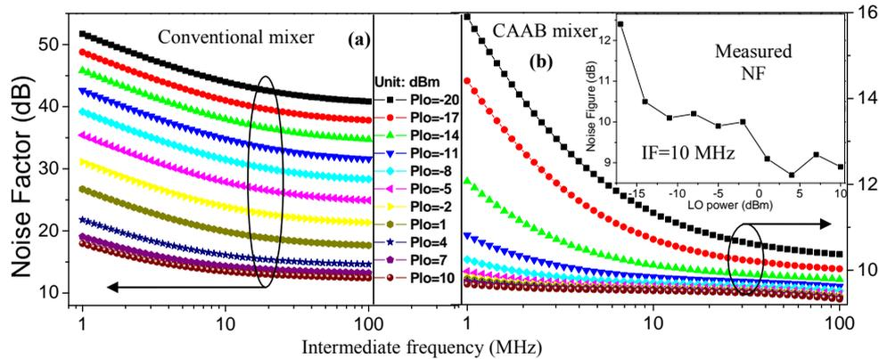
**Figure 10.** Noise figures at different  $LO$  input power. (a) Conventional mixer; (b) DBGC CAAB mixer; inset: measured  $NF$  at  $IF = 10$  MHz.
