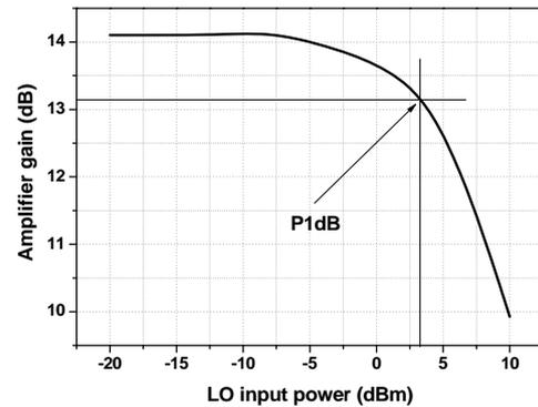
**Figure 6.** The simulated voltage gain of the Amp.
