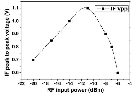
**Figure 13. IF peak-to-peak voltage versus RF input power. (The result is measured with the termination of oscilloscope at IF port).**
