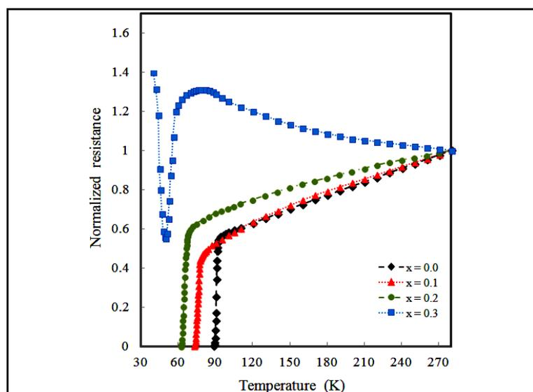
**Figure 3.** Variation of normalized resistance with temperature of  $Y_1Ba_2Cu_{3-x}Pr_xO_{7-\delta}$  samples with  $x = 0.0, 0.1, 0.2,$  and  $0.3$ .
