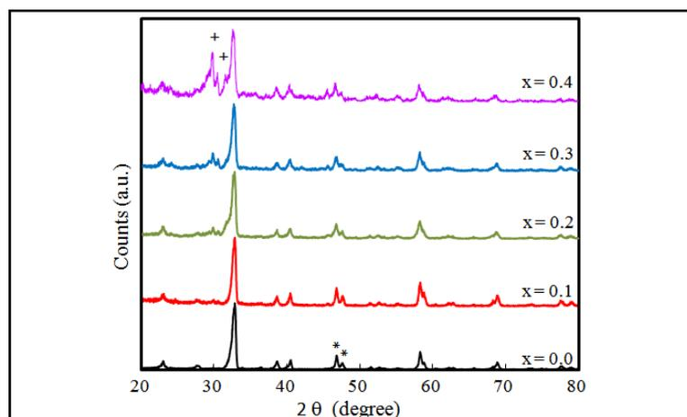
**Figure 2.** Normalized XRD pattern of  $Y_1Ba_2Cu_{3-x}Gd_xO_{7-\delta}$  samples with  $x = 0.0, 0.1, 0.2, 0.3,$  and  $0.4$ . The peaks denoted by (+) referred to  $Y_2BaCuO_5$  phase while (\*) peaks referred to (020) and (200) indices.
