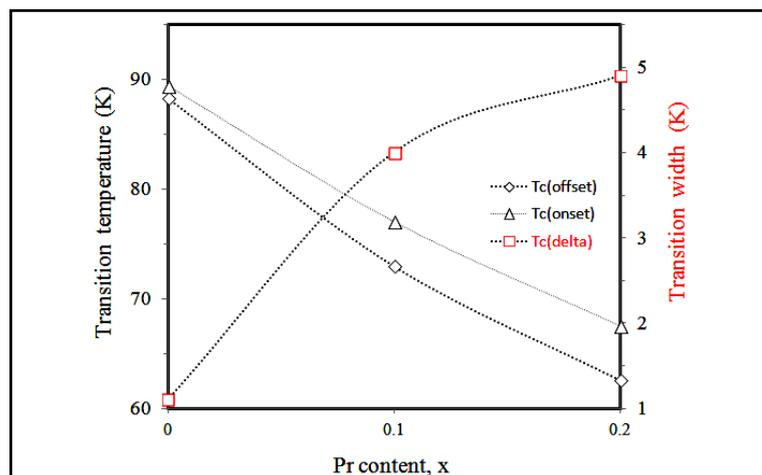
**Figure 4.** Dependence of the critical transition temperatures and transition width on Pr-content,  $x$ .
