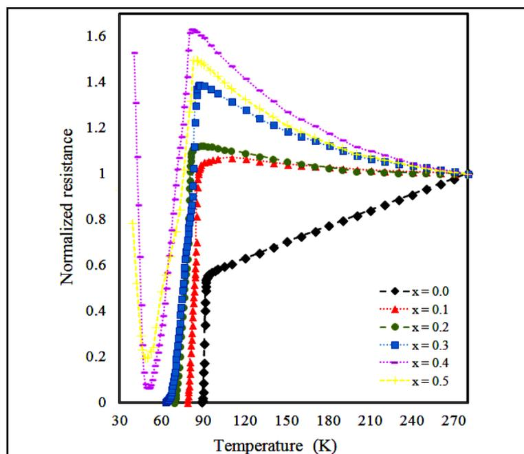
**Figure 5.** Variation of normalized resistance with temperature of  $Y_1Ba_2Cu_{3-x}Gd_xO_{7-\delta}$  samples with  $x = 0.0, 0.1, 0.2, 0.3, 0.4,$  and  $0.5$ .
