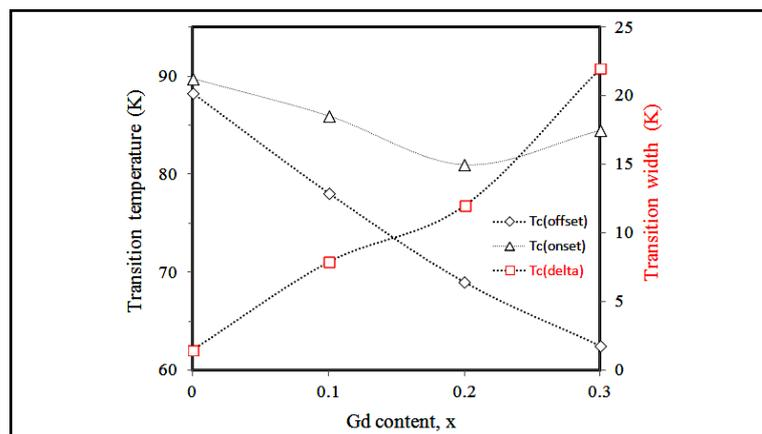
**Figure 6.** Dependence of critical transition temperatures and transition width on Gd-content,  $x$ , of prepared  $Y_1Ba_2Cu_{3-x}Gd_xO_{7-\delta}$  samples.
