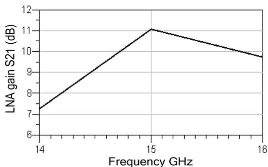
Figure 6. Simulated LNA output gain.
