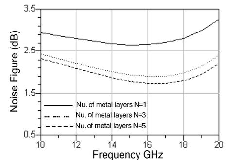
**Figure 5. LNA noise figure versus frequency with different layers of on-chip inductor ( $N = 1, 3,$  and  $5$ ) for  $C_p = 120$  pF.**
