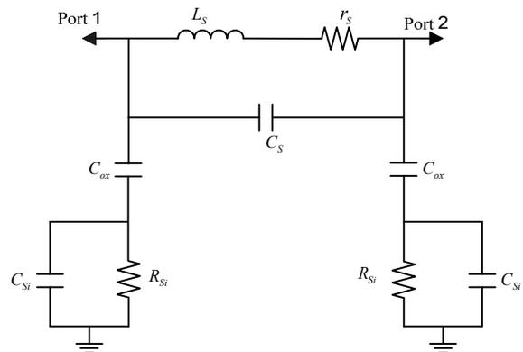
**Figure 2.** Lumped model of spiral inductor.
