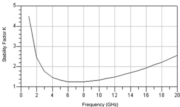
Figure 9. LNA Circuit Stability Factor  $K$  versus frequency.
