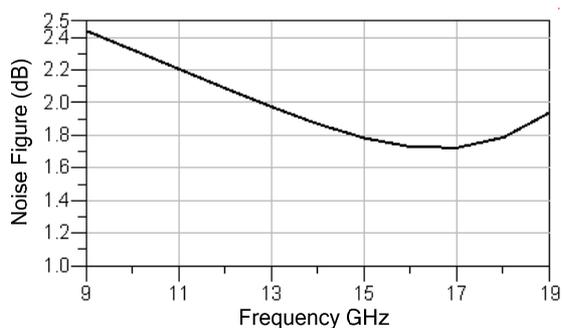
Figure 8. Simulated LNA noise figure.
