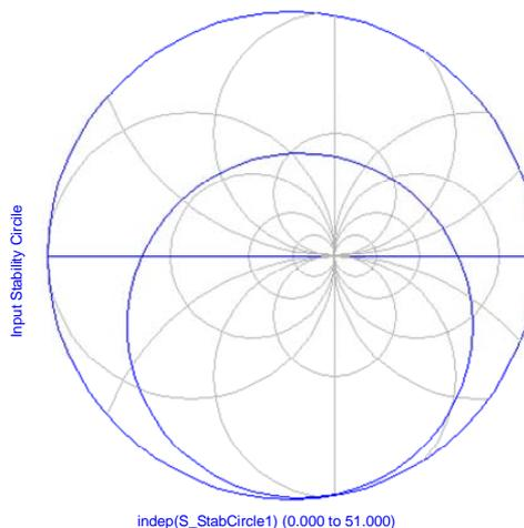
Figure 10. LNA input stability circle.
