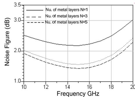
**Figure 4. LNA noise figure versus frequency with different layers of on-chip inductor ( $N = 1, 2,$  and  $3$ ) for  $C_p = 0$ .**
