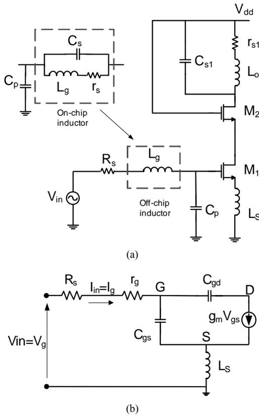
**Figure 1.** (a) Schematic circuit diagram of the proposed CMOS LNA; (b) Small-signal equivalent circuit.
