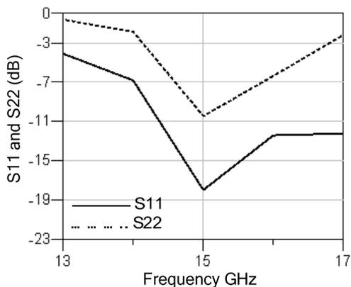
Figure 7. Simulated LNA input and output matching.
