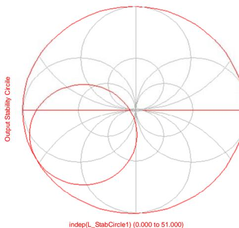
Figure 11. LNA output stability circle.
