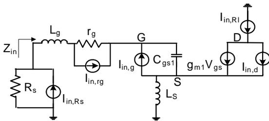
**Figure 3. Circuit model for input stage noise analysis.**
