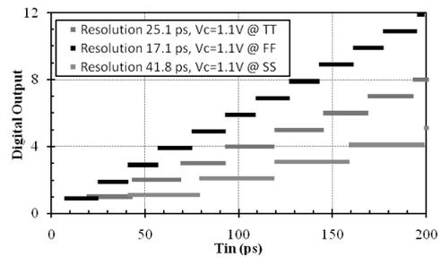
Figure 18. Variability of the digital output characteristics of the single-stage VTDC with the dynamic-logic phase detector as a function of process variations (in the TT, FF, and SS process corners), for a constant control voltage,  $V_c = 1.10$  V. Only the 0 - 200 ps fraction of the time scale has been shown for simplicity. (A small vertical offset in the digital output has been introduced for better readability).
