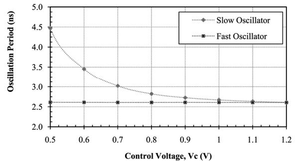
Figure 7. Oscillation periods of the voltage-controlled oscillators versus control voltage.
