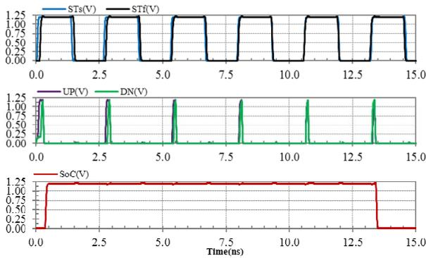
**Figure 12. Timing diagram of dynamic-logic phase detector.**
