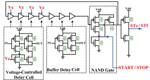
Figure 6. Schematic of the triggerable voltage-controlled oscillator.
