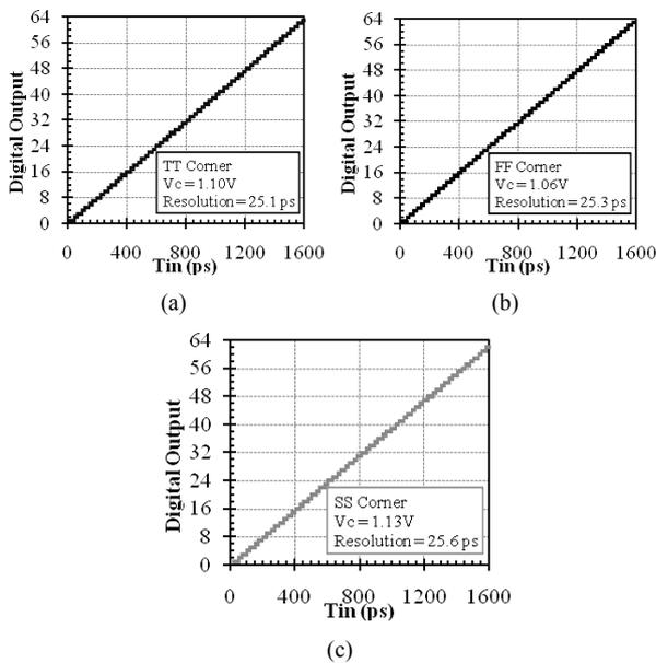
**Figure 19. Digital output characteristics of the single-stage VTDC with the dynamic-logic phase detector in the different process corners compensated using different values of the control voltage (a) TT corner,  $V_c = 1.10V$ ; (b) FF corner,  $V_c = 1.06V$ ; (c) SS corner,  $V_c = 1.13V$ .**
