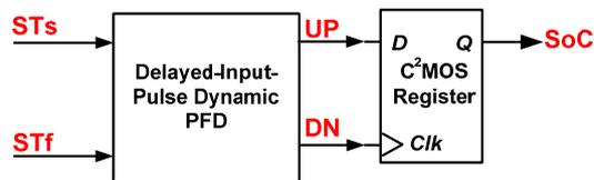
Figure 8. Dynamic-logic phase detector.
