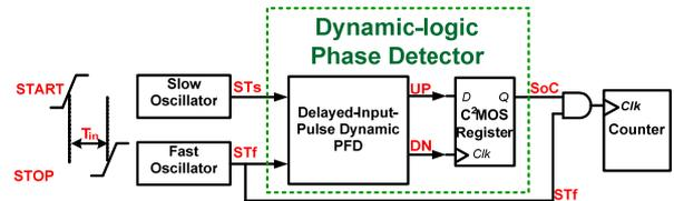
Figure 4. Single-stage VTDC with dynamic-logic phase detector.
