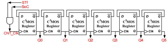
**Figure 13. Block diagram of the 6-bit counter.**
