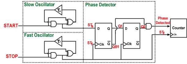
**Figure 2. Single-stage VTDC with a classic two-register phase detector [4].**
