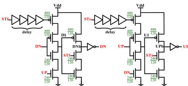
Figure 9. Delay-input-pulse phase frequency detector [11].
