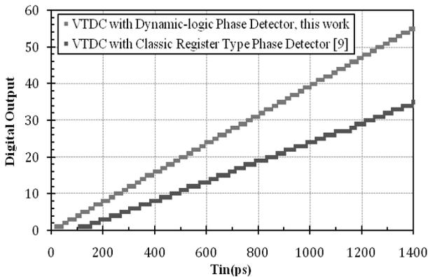
Figure 16. Comparison of the digital output characteristics of the single-stage VTDC with the dynamic-logic phase detector with the characteristics of the single-stage VTDC with the classic register-type phase detector from [6].
