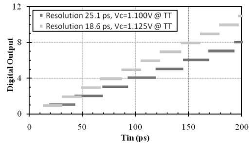
Figure 17. Digital output characteristics of the single-stage VTDC with the dynamic-logic phase detector in which the control voltage has been used to set up different time measurement resolution. Only the 0 - 200 ps fraction of the entire time scale has been shown for simplicity. (A small vertical offset in the digital output has been introduced for better readability).
