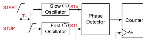
Figure 1. Concept of a single-stage Vernier Time-to-Digital Converter [4].
