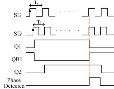
**Figure 3. Timing diagram of the correct phase detection [4].**
