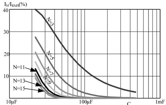
**Figure 15.** Theoretical values of the amplitudes of the line current harmonics for different capacitance values.
