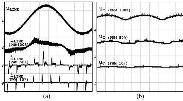
**Figure 23.** (a) Input AC line voltage,  $u_{LINE}$  (50 V/div), input AC line current,  $i_{LINE}$  (1 A/div), for different PWM dimming ratios (100%, 50% and 10%); time 2 ms/div. (b) DC link capacitor voltage,  $u_C$  (50 V/div), for different PWM dimming ratios (100%, 50% and 10%); time 2 ms/div.
