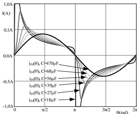
**Figure 13.** Theoretical waveforms of the AC line input current,  $i_{IN}$ , as a function of different capacitance values.
