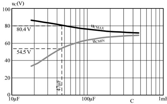
**Figure 17. Theoretical value of the peak (maximum) and valley (minimum) voltage values in a line period at capacitor  $C$  for different capacitance values.**
