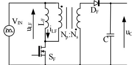
Figure 5. Schematics of the flyback input stage.
