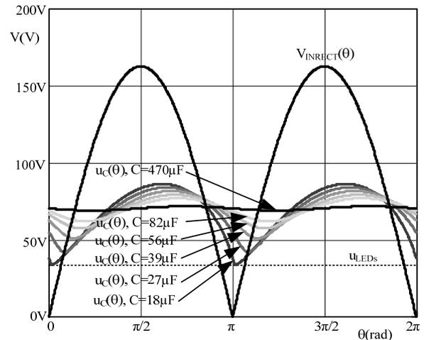
**Figure 12.** Theoretical waveforms of the capacitor voltage,  $u_c$ , as a function of different capacitance values.
