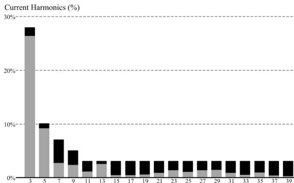
**Figure 20. Experimental harmonics of the input current of the integrated ballast for the selected value of  $47 \mu\text{F}$  (grey), and current harmonic limits given by IEC 61000-3-2 (black)**
