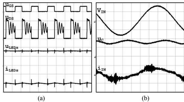
**Figures 25.** Experimental waveforms for 50% AM dimmed operation of converter (AM dimming 50%). (a) Gate to source voltage,  $U_{GS}$  (20 V/div); drain to source voltage,  $U_{DS}$  (200 V/div); LEDs forward current,  $i_{LEDs}$  (500 mA/div) and LEDs voltage,  $u_{LEDs}$  (20 V/div); time 5  $\mu$ s/div; (b) Input AC line voltage,  $u_{LINE}$  (50 V/div), input AC line current,  $i_{LINE}$  (500 mA/div), DC link capacitor voltage,  $u_C$  (50 V/div); time 2 ms/div.
