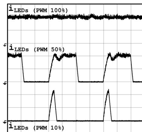
**Figure 22. Experimental waveforms of the current through the LEDs for PWM dimmed operation of converter (PWM dimming 100%, 50% and 10%). All traces 500 mA/div, 500  $\mu\text{s}$ /div.**
