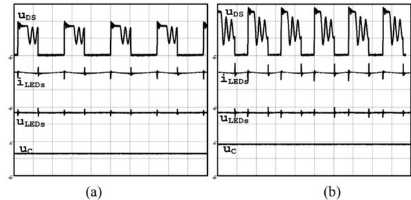
**Figure 18. Main experimental high frequency waveforms in the built prototype, at different line angles. (a)  $V_{IN} = 100 \text{ V}$  ( $\theta \approx 50^\circ$ ). (b)  $V_{IN} = 162 \text{ V}$  ( $\theta \approx 90^\circ$ ). (all traces:  $u_C$  50 V/div;  $u_{LEDs}$ : 20 V/div;  $u_{DS}$ : 200 V/div,  $i_{LEDs}$ : 500 mA/div; time: 5  $\mu\text{s}$ /div).**
