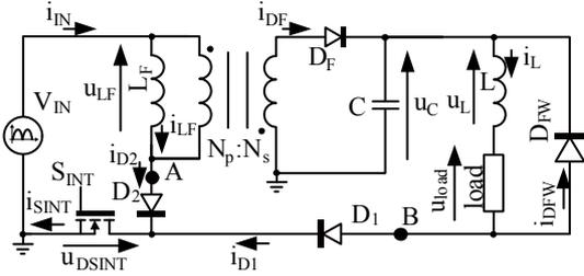
Figure 8. Full ballast with the integration of the stages.
