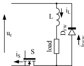
**Figure 3. Scheme of the output stage**
