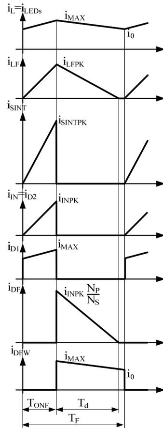
Figure 10. Main current waveforms at the proposed topology.
