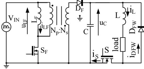
Figure 7. Full ballast with the proposed stages.
