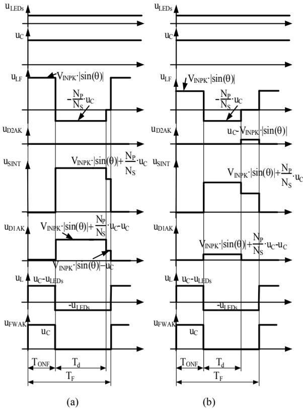
**Figure 11. Main voltage waveforms at the proposed topology. (a) High line instant input voltage condition. (b) Low line instant input voltage condition.**
