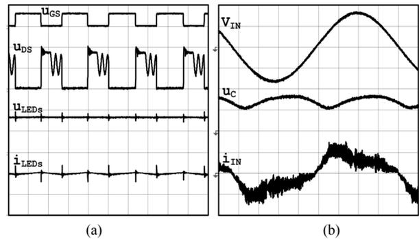
**Figures 24.** Experimental waveforms for full power operation of converter (AM dimming 100%). (a) Gate to source voltage,  $U_{GS}$  (20 V/div); drain to source voltage,  $U_{DS}$  (200 V/div); LEDs forward current,  $i_{LEDs}$  (500 mA/div) and LEDs voltage,  $u_{LEDs}$  (20 V/div); time 5  $\mu$ s/div; (b) Input AC line voltage,  $u_{LINE}$  (100 V/div), input AC line current,  $i_{LINE}$  (500 mA/div), DC link capacitor voltage,  $u_C$  (50 V/div); time 2 ms/div.
