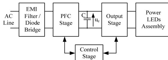
**Figure 1.** Block diagram of an offline electronic driver for Power LEDs.
