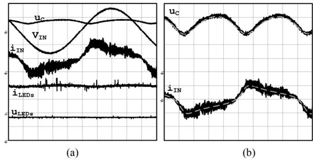
**Figure 19. (a) Main experimental line frequency waveforms ( $u_C$  and  $u_{LEDs}$ : 50 V/div;  $u_{RECT}$ : 100 V/div;  $i_{LEDs}$ : 1 A/div;  $i_{IN}$ : 500 mA/div; time: 2 ms/div); (b) Comparison between theoretical and experimental waveforms of  $u_C$  and  $i_{IN}$  ( $u_C$  20 V/div;  $i_{IN}$ : 500 mA/div; time: 2 ms/div).**
