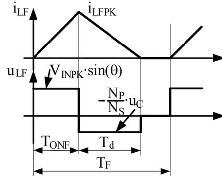
**Figure 6.** Main waveforms in the magnetizing inductor at the primary side of the transformer of the input stage.
