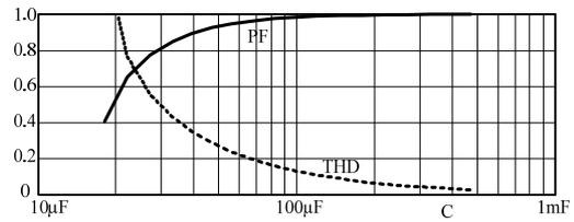
**Figure 14.** Theoretical values of  $PF$  (filled line) and THD (dotted line) of the input current, for different  $C$  values.
