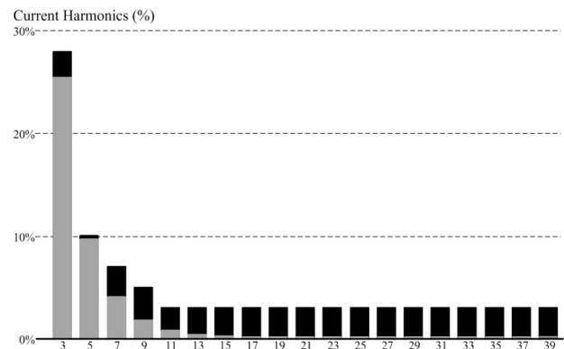
**Figure 16.** Theoretical harmonics of the input current of the integrated ballast for the selected value of  $47 \mu F$  (grey), and current harmonic limits given by IEC 61000-3-2 (black).
