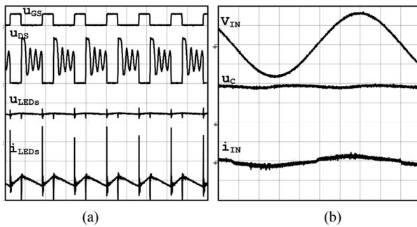
**Figures 26. Experimental waveforms for 10% AM dimmed operation of converter (AM dimming 10%). (a) Gate to source voltage,  $U_{GS}$  (20 V/div); drain to source voltage,  $U_{DS}$  (200 V/div); LEDs forward current,  $i_{LEDs}$  (200 mA/div) and LEDs voltage,  $u_{LEDs}$  (20 V/div); time 5  $\mu$ s/div; (b) Input AC line voltage,  $u_{LINE}$  (50 V/div), input AC line current,  $i_{LINE}$  (500 mA/div), DC link capacitor voltage,  $u_C$  (50 V/div); time 2 ms/div.**
