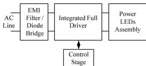
**Figure 2. Block diagram of an integrated electronic driver for Power LEDs.**
