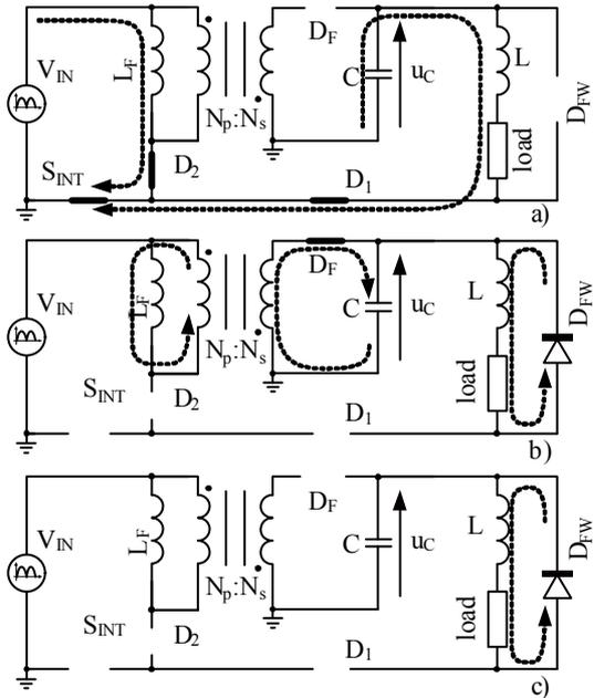
Figure 9. Switching modes of the integrated proposed driver.
