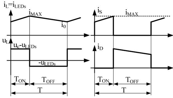
Figure 4. Main waveforms at the buck converter.
