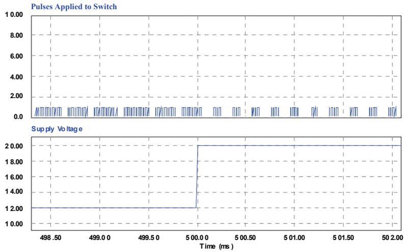
Figure 4. Increased pulse skipping with input voltage increase.
