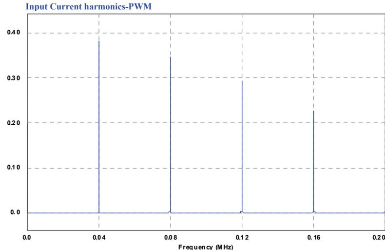
Figure 8. Input current harmonic spectrum – PWM converter.
