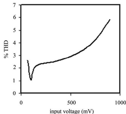
Figure 7. Variation of THD with input signal amplitude.
