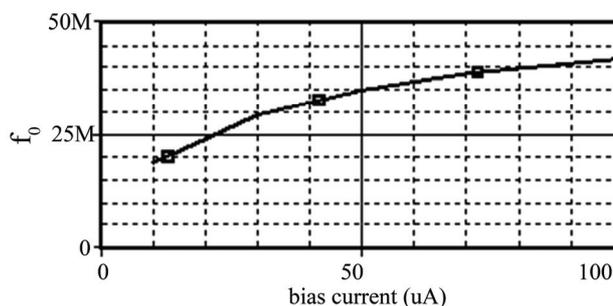
Figure 6. Dependence of central frequency on bias current.
