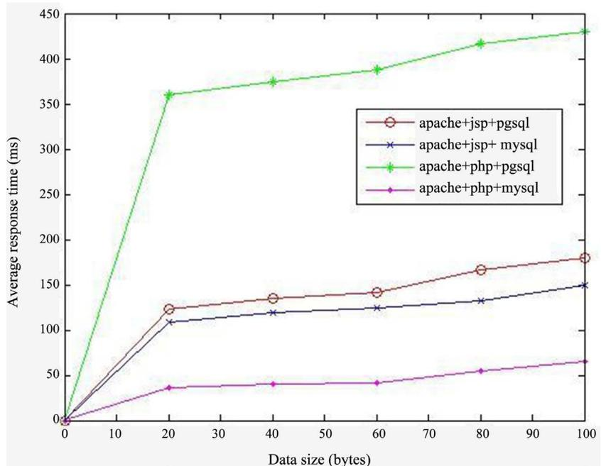
Figure 7. Average time response depending on the size of the retrieved data in the 4<sup>th</sup> column.
