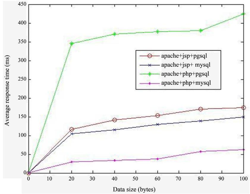
Figure 6. Average time response depending on the size of the retrieved data in the 3<sup>th</sup> column.
