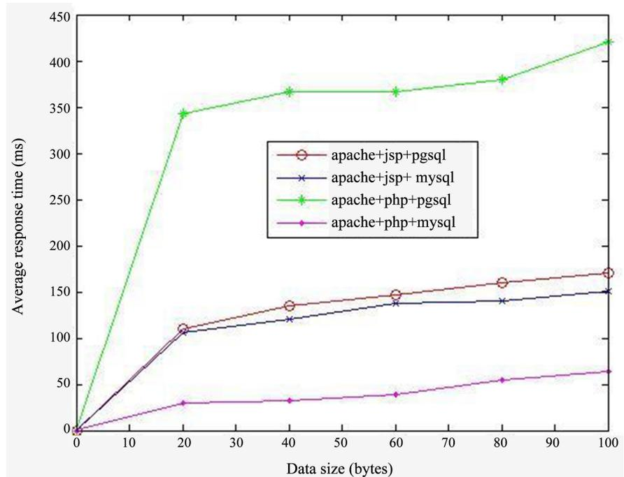
**Figure 5.** Average time response depending on the size of the retrieved data in the 2<sup>nd</sup> column.
