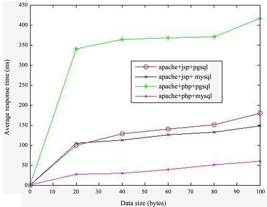
**Figure 4.** Average time response depending on the size of the retrieved data in the 1<sup>st</sup> column.
