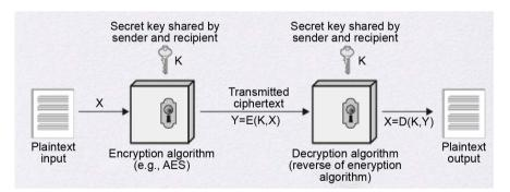
Figure 14. Cryptography symmetric encryption [3].
