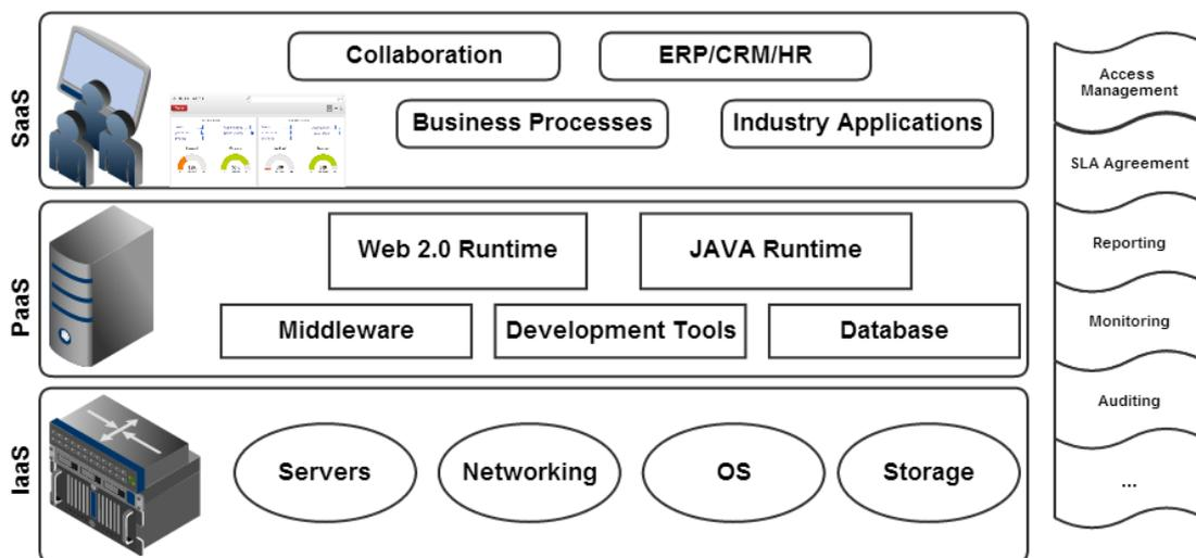
Figure 3. Cloud computing delivery models (adapted from [8,12,19]).
