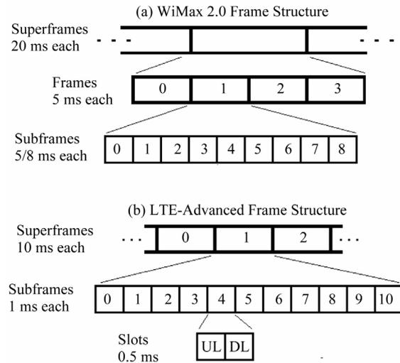
**Figure 2. Frame (a) WiMAX 2.0; (b) LTE-Advanced.**
