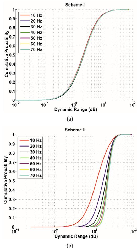
**Figure 1.** The cumulative probability of the channel's dynamic range  $D$  over a fountain-encoded packet: the transmission **Scheme I** (top) and the transmission **Scheme II** (bottom). (a) Transmission **Scheme I**; (b) Transmission **Scheme II**.
