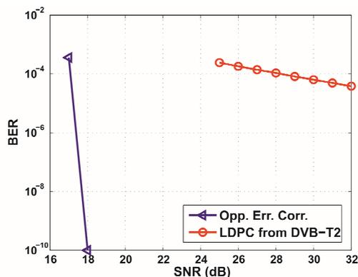
**Figure 4.** BER comparison between opportunistic error correction and the (7200, 16200) LDPC code from the DVB-T2 standard in the noisy TU6 channel with perfect channel estimation. For opportunistic error correction, no error occurs when SNR  $\geq 18$  dB. So for this point, we represent BER = 0 by  $10^{-10}$ .
