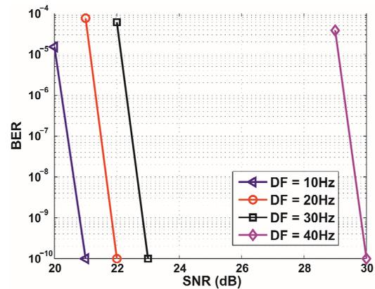
**Figure 6. BER performance of opportunistic error correction in the noisy TU6 channel with the non-perfect channel estimation. For  $DF = 10$  Hz, no error occurs at SNR = 21 dB. So for this point, we represent BER = 0 by  $10^{-10}$ . Same for  $DF = 20 - 40$  Hz.**
