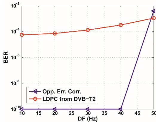
**Figure 5. BER comparison between opportunistic error correction and the FEC layer in the DVB-T2 standard in the noiseless TU6 channel with the non-perfect channel estimation. For opportunistic error correction, no error occurs when DF = 10 - 40 Hz. So for those points, we represent BER = 0 by  $10^{-10}$ .**
