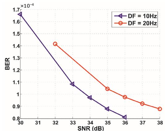
**Figure 7. BER performance of the (7200, 16200) LDPC code from the DVB-T2 standard in the noisy TU6 channel with the non-perfect channel estimation.**
