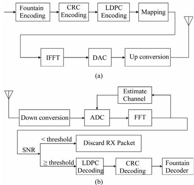
**Figure 2. Proposed DVB-T2 transmitter (top) and receiver (bottom). (a) Transmitter; (b) Receiver.**
