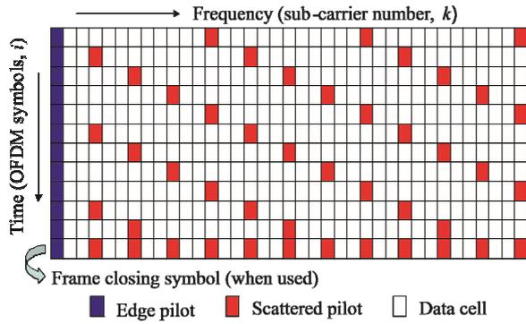
Figure 3. Scattered pilot pattern PPI (SISO) [5].
