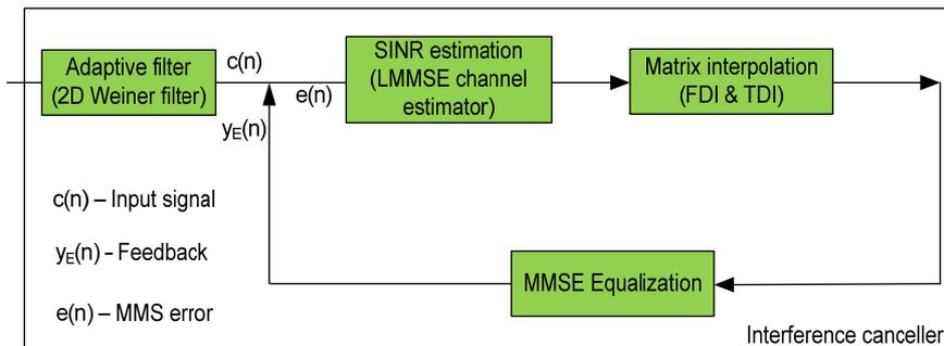
Figure 2. Proposed Iterative model for MIMO receiver.
