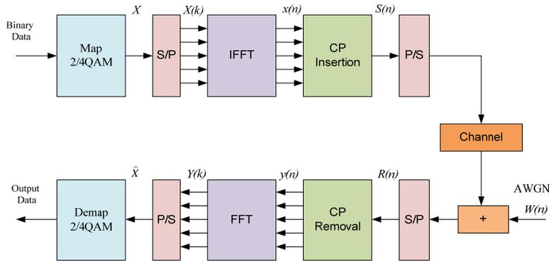
Figure 1. The block diagram of an OFDM system.
