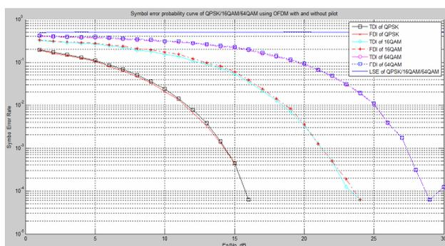
**Figure 6.** The symbol error rate comparison of the proposed non-pilot and pilot technique with any modulation order at the receiver.
