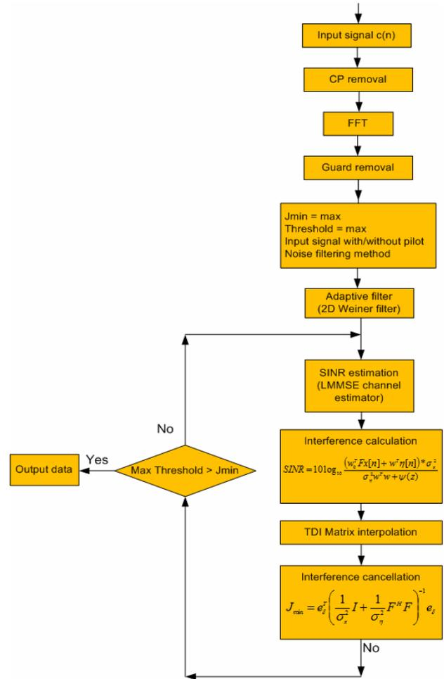
Figure 4. Proposed combination signal processing technique of ICS for 3GPP/LTE.
