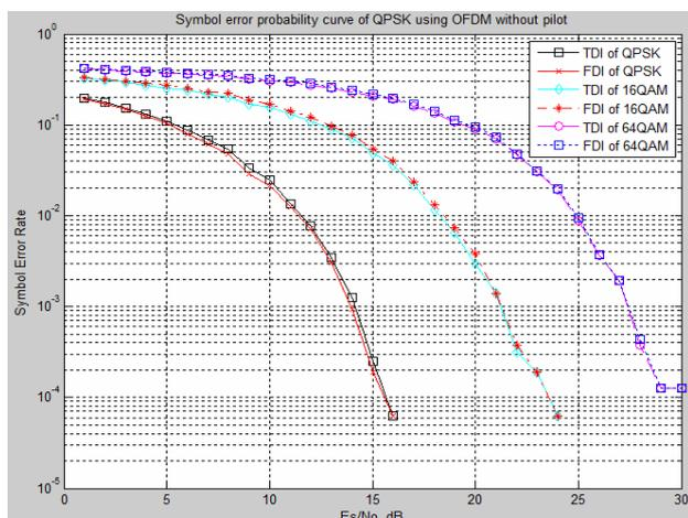
**Figure 5.** The symbol error rate comparison of the proposed non-pilot technique with that of a 2Tx–2Rx at the MMSE receiver.
