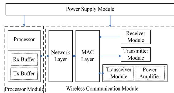
**Figure 3.** The structure of area controller.
