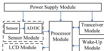
**Figure 2.** The structure of Electronic Intelligent Tag (EIT).
