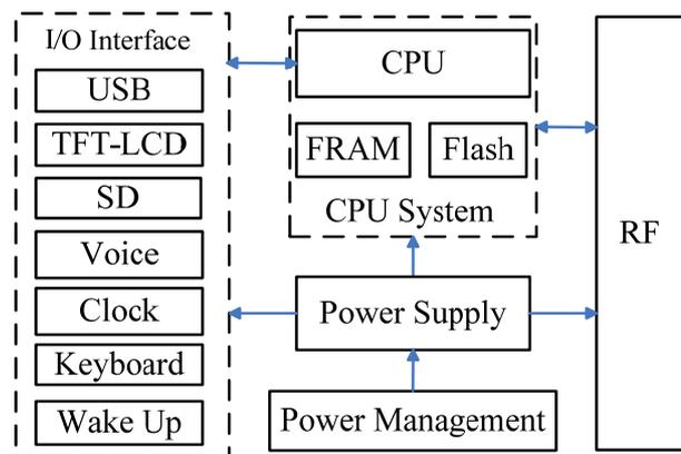
**Figure 5.** The structure of handheld instrument.
