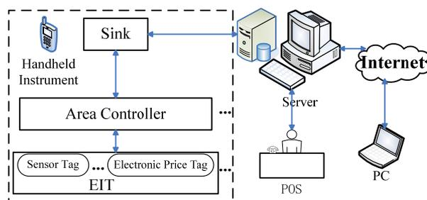
Figure 1. Architecture of Electronic Intelligent Tag System (EITS).
