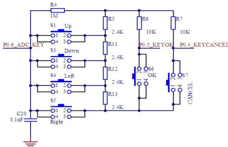
Figure 3. Switch control circuit.
