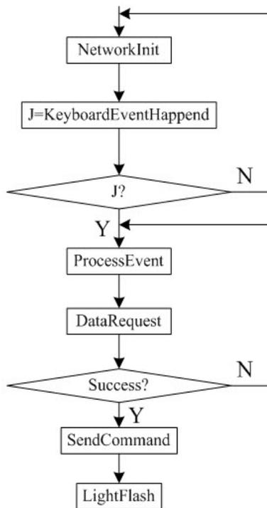
**Figure 7. Key light control algorithm.**
