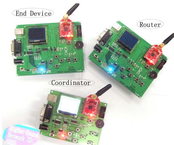
**Figure 8. Wireless light control networking.**
