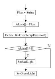
Figure 6. Over-temperature alarm.
