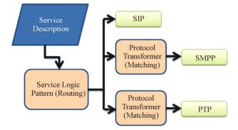
Figure 5. Service Protocol routing and matching.
