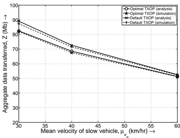
Figure 3. Aggregate data transferred vs mean velocity of slow station ( $\mu_{v_F} = 120$  km/hr and  $k_{jam} = 80$ ,  $\sigma_{v_S} = \sigma_{v_F} = 5$  km/hr).
