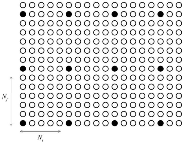
Figure 2. Pilot symbols in the OFDM signals.
