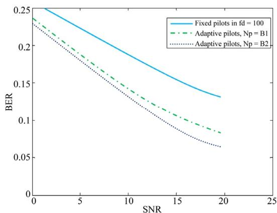
**Figure 7. BER performance of the OFDM system with fixed pilots and adaptive pilots based on obtained tight bound with  $N_p = B_1$  and  $N_p = B_2$ .**
