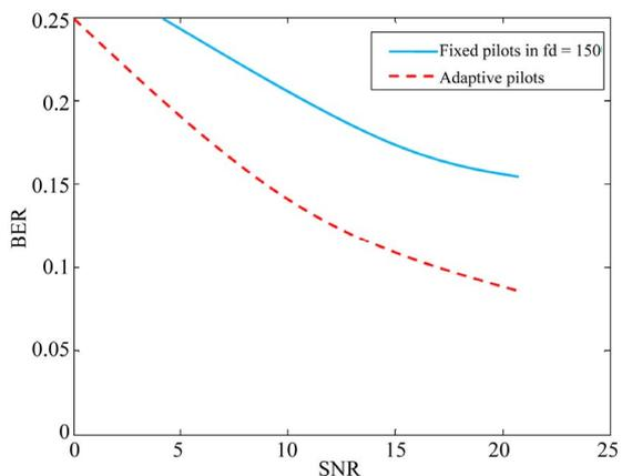
**Figure 6. Performance improvement using adaptive resource allocation based on the first lower bound for the number of pilots,  $N_p = 4KN_s f_d T_s \tau_m \Delta F$ . Channel estimation using fixed pilots is implemented in  $f_d = 150$  Hz.**
