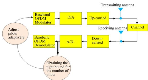
**Figure 3. Proposed OFDM system with adaptive scheme for number of used pilots.**
