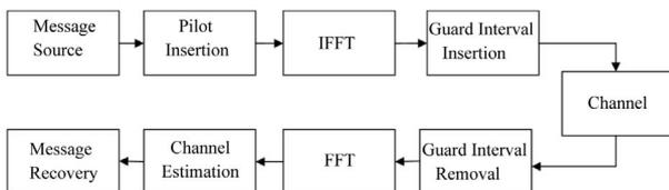
**Figure 1. Baseband OFDM transceiver.**
