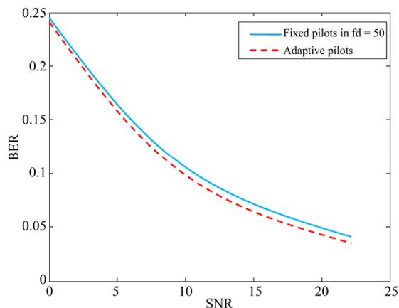
**Figure 5. Performance improvement using adaptive resource allocation based on the first lower bound for the number of pilots,  $N_p = 4KN_s f_d T_s \tau_m \Delta F$ . Channel estimation using fixed pilots is implemented in  $f_d = 50$  Hz.**
